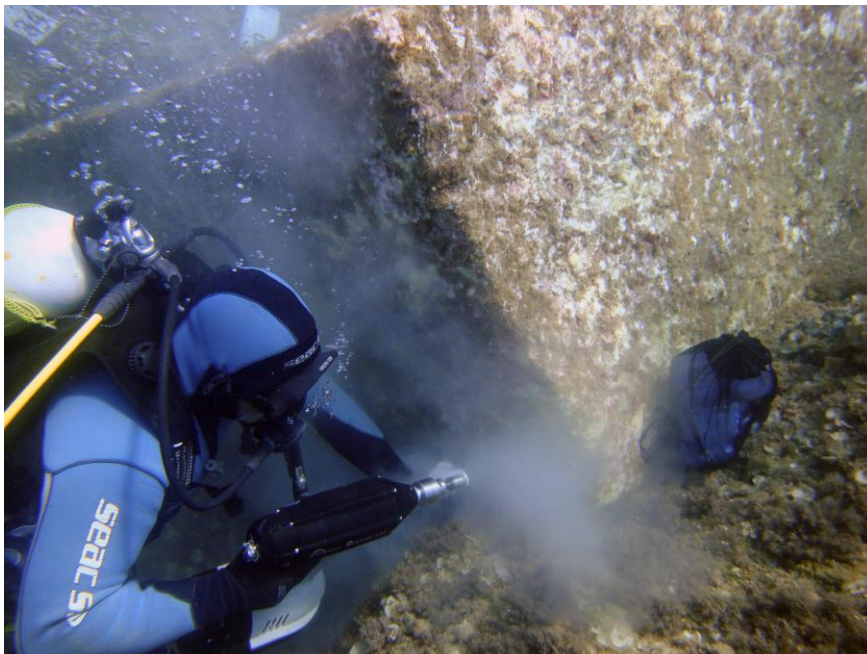
Fig. 7. Cala Cicala. Sampling with an underwater mechatronic drill (from Antonelli et al. 2000; photo by S. Medaglia).
